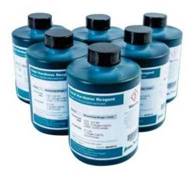
The hardness reagents are only suitable for use with the LSW-JP-TH instruments, which measure different water hardness ranges by selecting different types of reagents.
